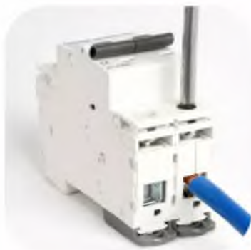
Safety terminal: easy wiring; protection degree IP20. Pozidriv and slot screw head. Torque up to 2.8 N·m.
